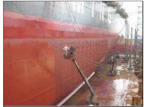
When spraying, keep about 1 m wide spray shift at right angle
