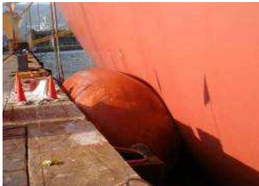
Flexible fender / sprinkling water to hull
