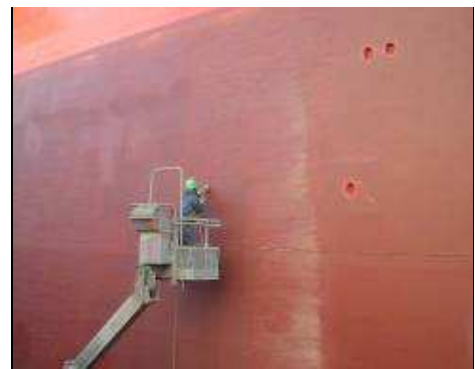
Dust removal by power tool
