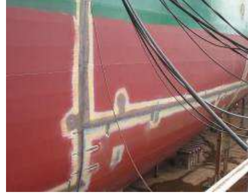
Surface preparation of erection joints (Power tool cleaning)
