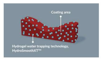
The Nippon Paint Marine team focused on replicating this natural phenomenon and developing specifically designed hydrogels for paints; the scientific theory being that a hull coating could be created that 'traps' a layer of seawater into the surface boundary membrane, which in turn, increases the more controlled turbulence generation of a vessel's hull, reducing friction.
